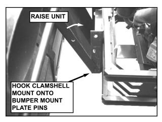
**STEP 13:** Hook bottom of clamshell mount onto pins in bottom of bumper mount plate, then raise clamshell assembly up against bumper mount.
